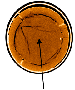
Chevron fracture due to damage in transit/handling
