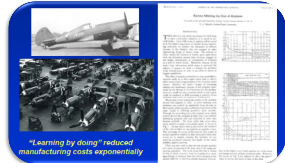
T.P. Wright (1936) found that the cost of making airplanes declined with increasing experience
