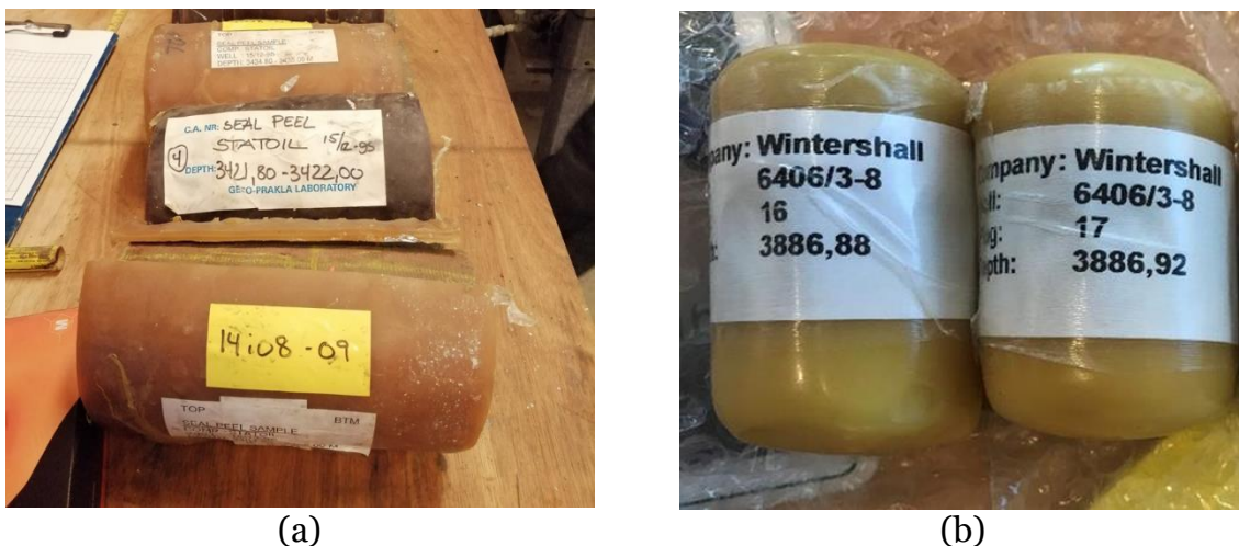
Figure 1. (a) Seal peels by wax dipping, (b) Preserved cores plugs with the film-foil-wax method
