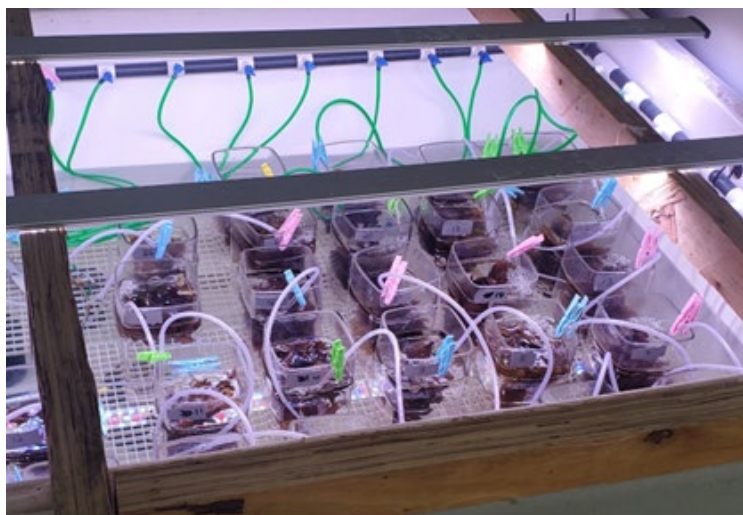
Figure 2: Water bath with 25 (5 treatments x 5 replicates) glass containers containing Palmaria palmata .
