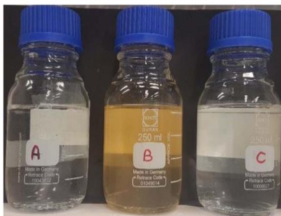
Fig. 5. Change in colour of the prepared FW (A) when stored in stainless steel (B) and titanium (C) piston cells respectively. The colour change in FW (B) can be attributed to corrosion formation resulting from the stainless-steel piston-cell coupled with the corrosive nature of the studied system. Since the prepared FW and the brine store in titanium piston-cell were both colourless (A and C respectively). It confirms that the corrosion challenge can be mitigated by using titanium piston-cell.
