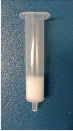
Figure 1: Syringe with frits used to filter emulsions.
