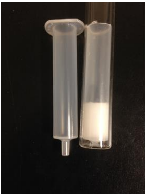
Figure 5.2.1: Syringe without silica plug (left) and modified syringe in NMR tube prepared with silica plug (right).
